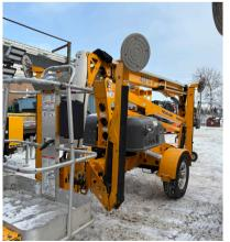
The compact and lightweight design makes them towable to any site, no CDL required. Hydraulic outriggers set-up in less than 30 sec for safe work on uneven ground.
